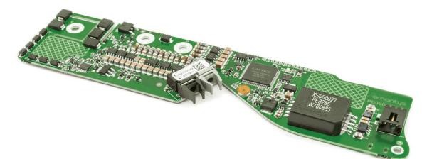
The 3300V, P Series On-module Gate Drive will drive high power single switch IGBT modules for 2-level and multi-level applications. The gate drive incorporates protection features for the IGBT module and can be configured by the user to optimise the operation of the gate drive in the power stack of the end application. 1200V and 1700V variants are also available.
